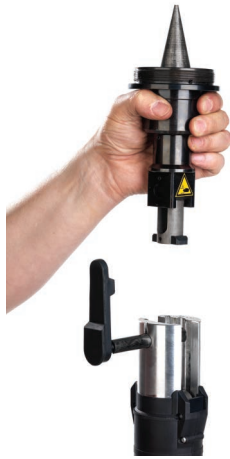
▲ Fig. 88: Mount the expander head on the drive unit.
