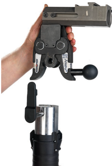
▲ Fig. 93: Click the clamping jaws on the compatible drive unit.
