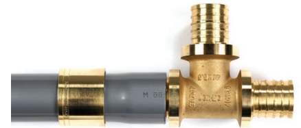
▲ Fig. 92: Push the fitting into the pipe. After a short period of time, the fitting has a tight fit in the pipe. (PEX has a larger "memory" effect than STABIL).
