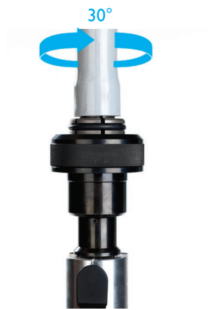
▲ Fig. 91: Operate the drive unit. The pipe is widened. Repeat this at least twice (turn by 30°).
