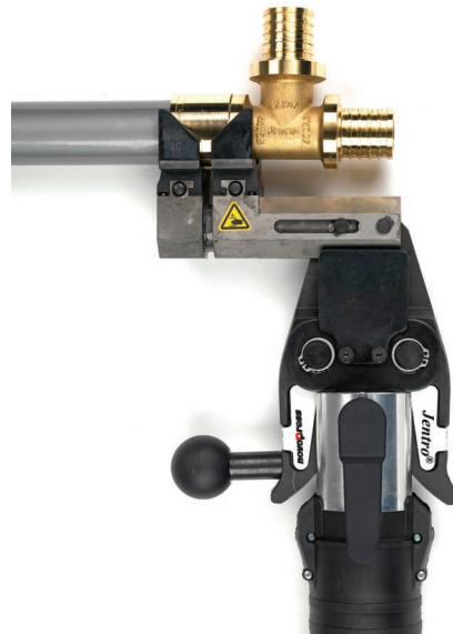
▲ Fig. 94: Operate the drive unit to push the compression sleeve right up to the fitting collar. Both clamping heads are identical.
