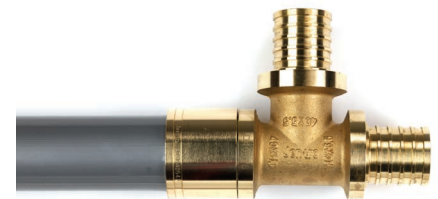
▲ Fig. 95: Compression joint ready. Sleeve right up to the flange edge.
